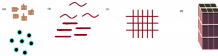
Fig. 1 Different dimensional Nanomaterials (a) 0-D spheres and clusters, (b) 1-D nanofibers, wires, and rods, (c) 2-D films, networks, (d) 3-D nanomaterials.
